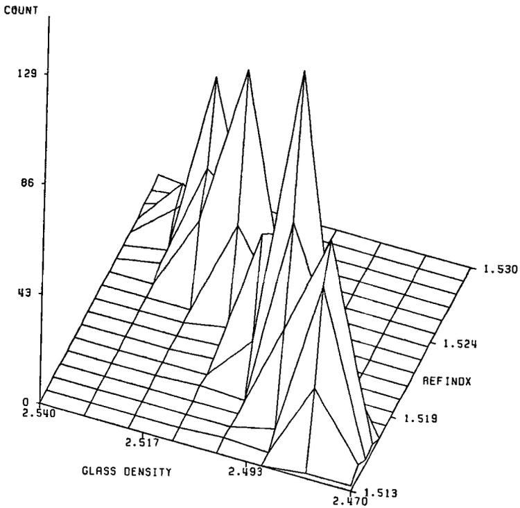
FIG. 2—Three-dimensional representation of glass density and refractive index data. The data are the same as that depicted in Fig. 1, but the axes have been rotated by the SASGRAPH routines to display another projection.
