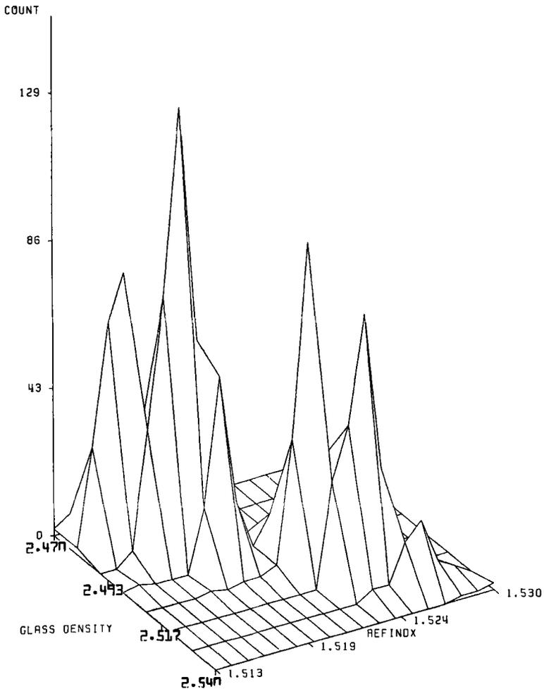
FIG. 1—Three-dimensional representation of density and refractive index values determined by the FBI Laboratory on 1054 samples of glass.
