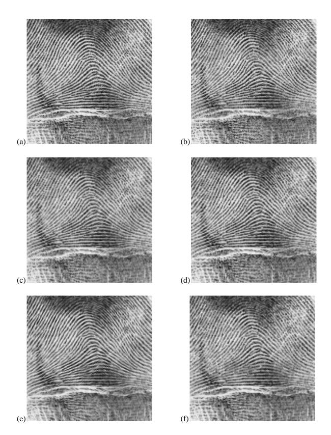
Figure 13. Interpolation results of the image Fingerprint. (a) Original Image; interpolated image by (b)Nearest Neighbor; (c) Bilinear; (d) Bicubic; (e) NEDI; (f) DFDF
