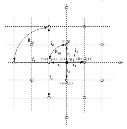
Figure 5. Geometric Duality when interpolating  $Y i_x j$  (i+j = odd) from  $Y i_x j$  (i+j = even) [4]
