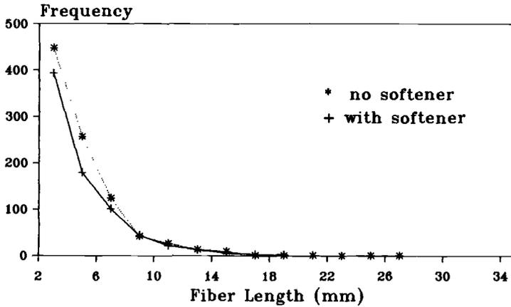
FIG. 7—Length distribution of fibers  $\geq 2$  mm transferred—woven MSL fabrics (A, B, C, and D).
