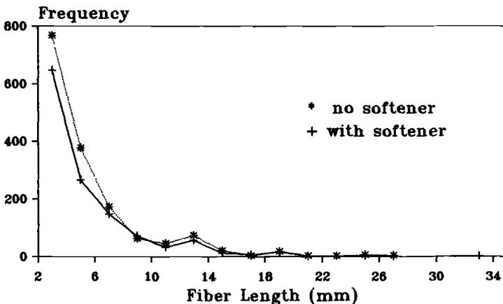
FIG. 4.—Length distribution of fibers  $\geq 2$  mm transferred—all fabrics (Fabrics A through I).
