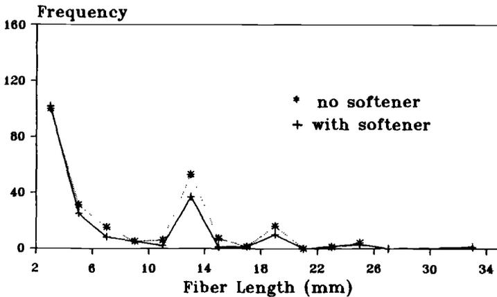
FIG. 8.—Length distribution of fibers  $\geq 2$  mm transferred—knit MSL fabrics (G and H).
