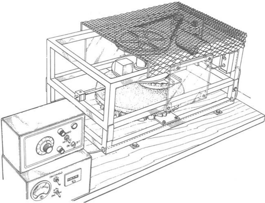
FIG. 1—Illustration of the fiber transfer abrasion tester (FTAT).
