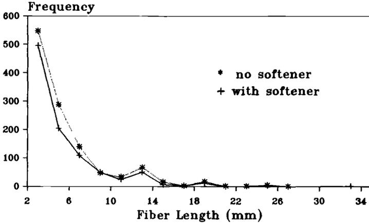
FIG. 6—Length distribution of fibers  $\geq 2$  mm transferred—all MSL fabrics (A, B, C, D, G, and H).
