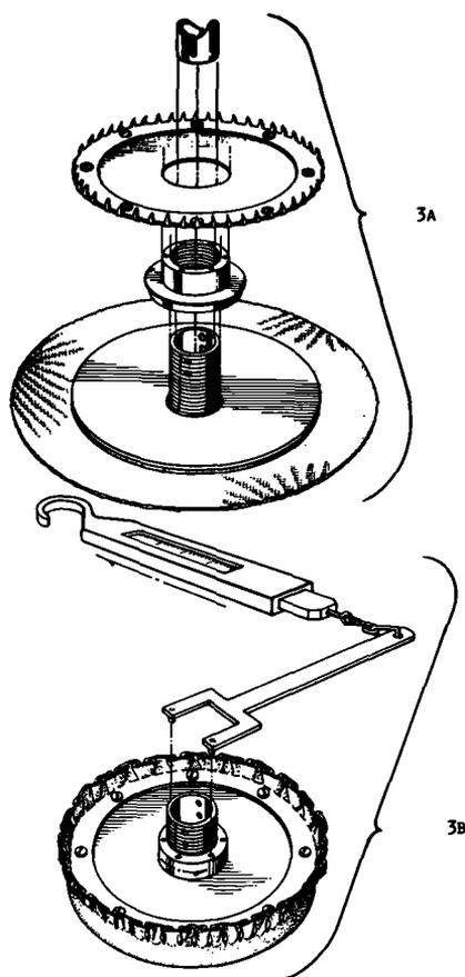
FIG. 3—Illustration showing attachment of fabric specimen to an abrasion pad; (a) before attaching fabric over hooks and (b) during torquing of fabric.
