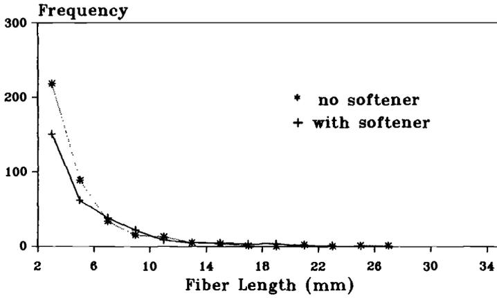
FIG. 5—Length distribution of fibers  $\geq 2$  mm transferred—non-MSL fabrics (E, F, and I).
